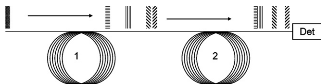
Fig. 1. In tandem serial column configurations, such as this, effluent from one stage flows directly to the next stage. Retention information relating to the first stage is not acquired. The retention information acquired relates to the net combination of both steps. In the illustration, 1st-dimension separation of horizontal and vertical striped peaks is degraded by subsequent passing through 2nd-dimension column.
